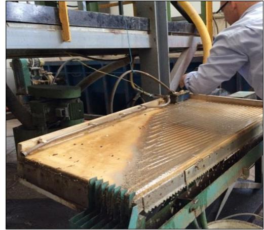
Figure 3: Separating a tungsten (scheelite) stream from Morille tailings using a shaker table.
