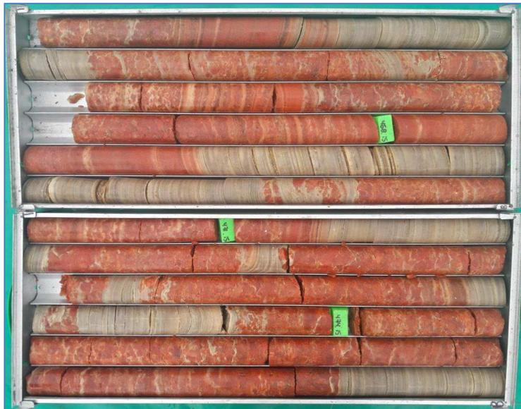
**FIGURE 1: CARNALLITE (PINK-RED) ZONES WITHIN HALITE SALT HORIZONS TYPICAL OF BROADER ZONES INTERSECTED IN BA003.**
