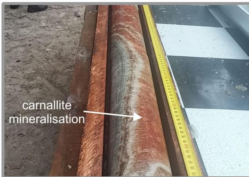
FIGURE 1: STEEPLY DIPPING, RED POTASH (CARNALLITE) MINERALISATION IN BA001
