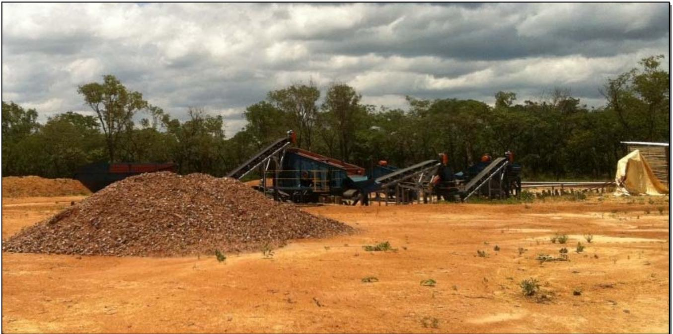
Figure 6: Stockpiled copper-gold bearing material at primary and secondary crusher location ready for transport to treatment facility on site 14923-HQ-SML.
